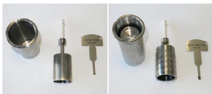
Figure 3. Coaxial cylinder geometry with profiled surface finish (left). Double gap measuring geometry with helical grooves.
