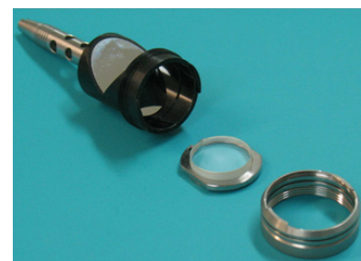
Figure 5: Upper measuring geometry consisting of a shaft with integrated mirror and a screw holder ring for mounting the exchangeable quartz glass plate, here with a circular quartz glass plate with 20 mm and steel clamp ring.
