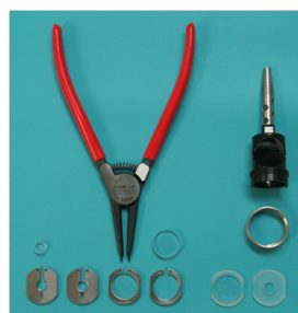
Figure 4: Accessories for the UV module: left: tool for spreading the glass plate clamps, clamps for circular glass plates with diameters of 8 and 20 mm, 8 and 20 mm circular glass plates with and without clamps, right: the one piece 8 and 20 mm plates glass, upper measuring geometry.
