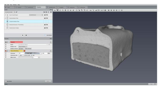
The *Recipes* panel allows the execution of user-defined recipes. Once a recipe is loaded into the panel, it can be played and edited. Multiple recipes can be loaded, and they can be saved on disk using a dedicated file format (hxrecipe).
