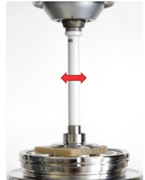
Figure 4: Measurement setup for amplitude and frequency (bulk) using a HAAKE MARS 60 Rheometer and plate-plate geometry P35.
