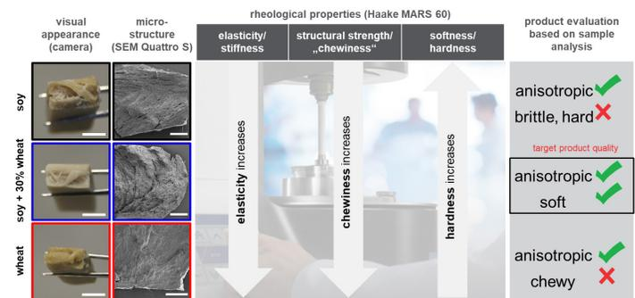
**Figure 9:** Evaluation of meat analog product quality based on sample analysis via optical and rheological tools.
