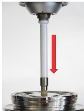
Figure 3: Measurement setup for compression tests using a HAAKE MARS 60 Rheometer and plate-plate geometry P8.
