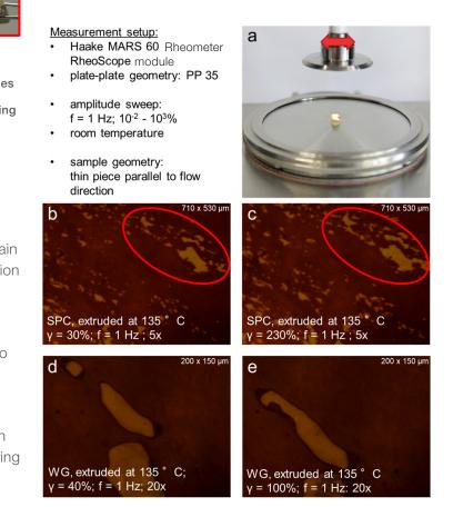
Figure 7: Change in micro-structure elements with increasing deformation, characterized by amplitude sweeps (thin layer) using a HAAKE MARS 60 Rheometer with RheoScope module and plate-plate geometry P35.
