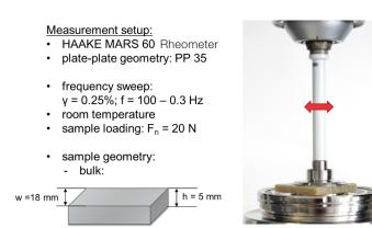
Figure 4: Measurement setup for amplitude and frequency (bulk) using a HAAKE MARS 60 Rheometer and plate-plate geometry P35.
