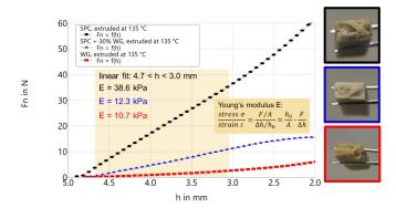
Figure 5: Change in the elasticity and stiffness of meat analog samples made from varying ratios of Soy Protein Concentrate (SPC) and Wheat Gluten (WG) characterized by compression analysis using a HAAKE MARS 60 Rheometer and plate-plate geometry P8.
