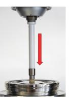
Figure 3: Measurement setup for compression tests using a HAAKE MARS 60 Rheometer and plate-plate geometry P8.
