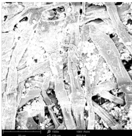
SEM image of paper imaged with no precaution (charging.)
