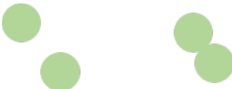
When spots are far enough apart to be distinguished, they are resolved. If they are too close, the edges will seem to overlap, and the objects will be unresolved.
