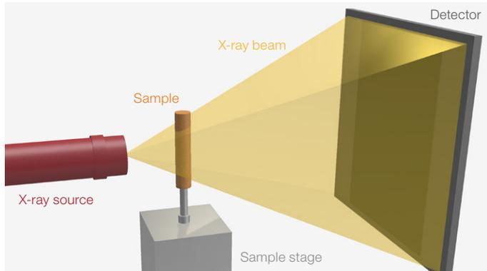
Figure 1. The microCT setup.
