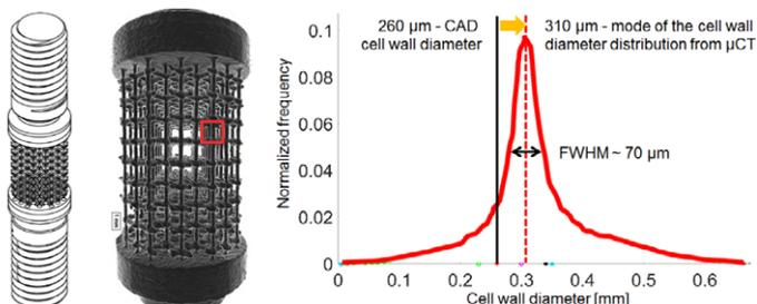
Figure 14. Showing left to right: CAD drawing of a Ti scaffold to aid bone growth; the resulting 3D scan post-imaging in the HeliScan microCT of the actual part; a graph of the column diameter taken at the red indicated square. [6]
