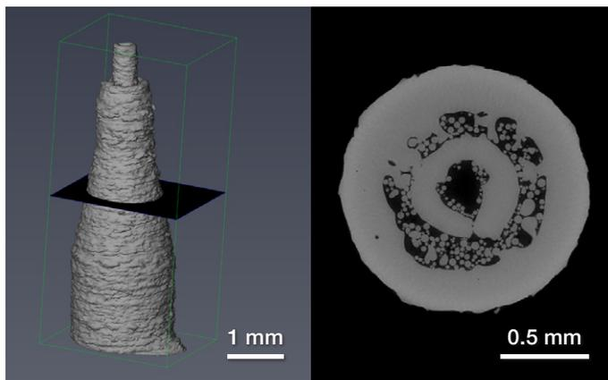
Figure 12. Slicing the 3D scanned object shows the inner wall broken allowing mixing to occur inside the injector. [6]
