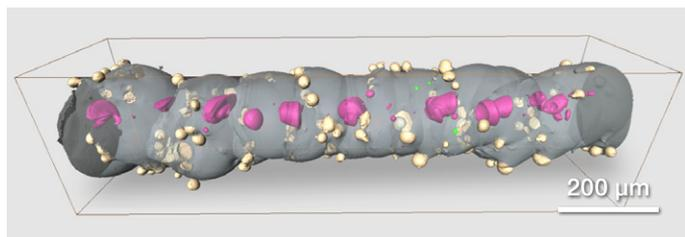
A part of a titanium additively manufactured scaffold.
