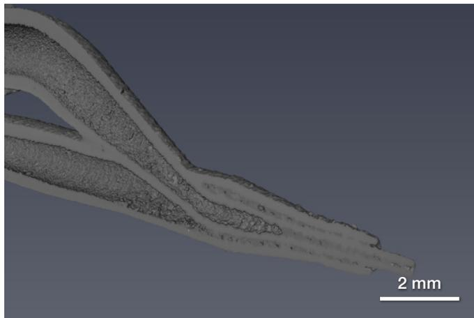
Figure 11. 3D image reconstruction of the injection system showing the structure. [6]
