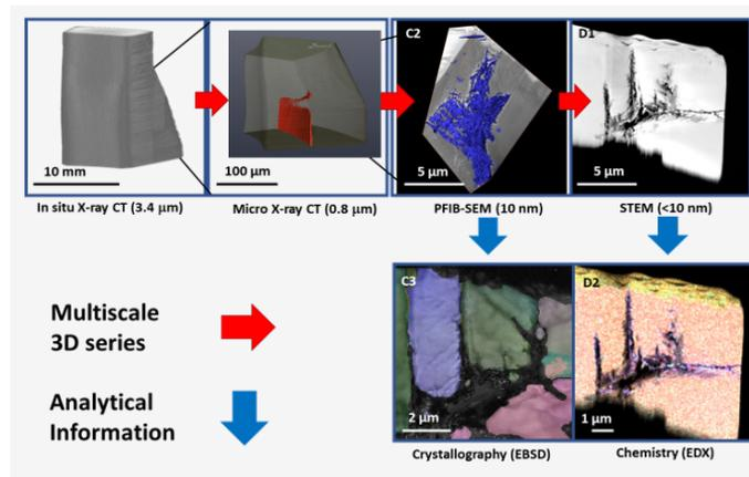
Figure 16. Stainless steel weld multi-scaled visualization from microCT to PFIB to TEM.
