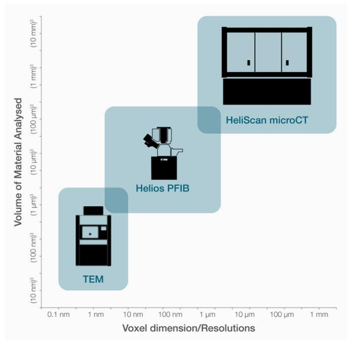
Figure 15. Typical analytical methods available in the modern laboratory.
