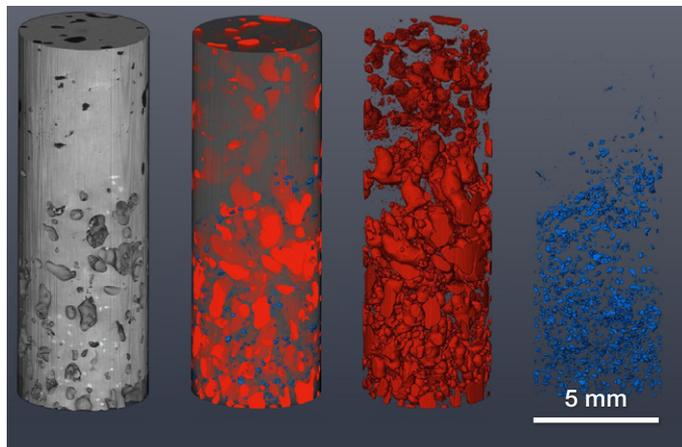
Figure 2. From left to right: A sample of CuAlZr alloy [6] X-ray image; surface-rendered X-ray image in red; the distribution of the pores within the sample in red; the dense particles in blue.
