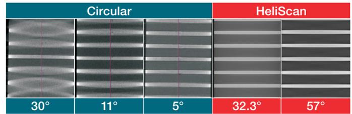
Figure 6. No distortion effects for the HeliScan microCT systems, unlike circular systems. [7]
