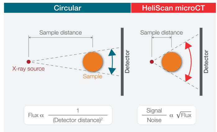
Figure 3. Low cone angle—Sample and detector far away from the source: low flux, low signal to noise ratio. High cone angle—Sample and detector closer to the source: high flux, improved signal to noise ratio. [7]
