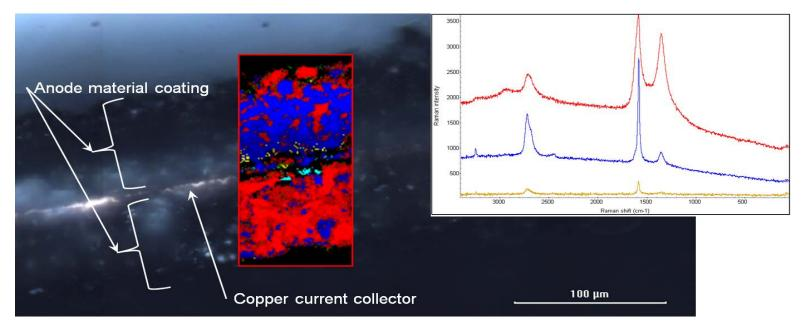
The red color indicates the presence of carbon black while the blue color represents graphite. The distribution of these materials on the two sides of the electrode is significantly different. The copper current collector is in the center.
