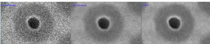
SEM image detail from a 3D NAND sample, acquired with a Thermo Scientific™ Helios™ 5 PXL Wafer DualBeam™ System, at a resolution of 1.22 nm per pixel. A short dwell time is used to prioritize acquisition throughput over signal-to-noise ratio. Left) raw image; middle) image denoised using the original N2V model; right) image denoised using the new N2V2 model, trained in the same conditions as the N2V image.
