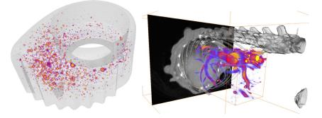
Illustration of Structure Enhancement Filter. Left: highlighting pores of varied sizes in aluminum cast. Right: highlighting blood vessels in small animal  $\mu$ CT.
