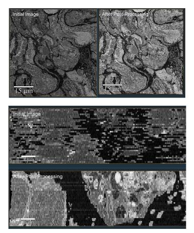
Figure 2: Comparison before and after post-processing with the EM Toolbox, performing contrast enhancement, linear, and elastic stack alignement. Top: in-plane comparison shows the contrast improvement using the same colormap, Bottom: cross-section comparison shows the effects of slice alignement. Data courtesy of Karol Malota, Department of Animal Histology and Embryology, Faculty of Biology and Environmental Protection, University of Silesia in Katowice
