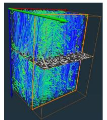
Figure 1: Fibers in Glass Fiber Reinforced Composite, visualized with Directionally Encoded Colors
