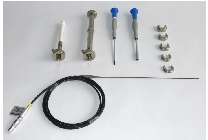
Figure 4: Solids clamping tool with temperature sensor, spacer and tool.
