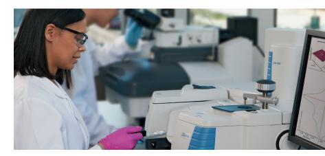
The Nicolet iS50R Spectrometer carries forward all the flexibility and performance of the Thermo Scientific™ Nicolet™ iS50 Spectrometer system, with the added capabilities for the research spectroscopist. The Nicolet iS50R includes dual sources and triple detector optics, multiple on-board digitizers and easy access to spectrometer data and control signals.
