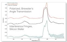
Improve sensitivity and surfaces and suppress interference with polarized measurements.
