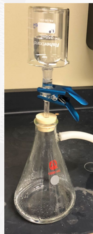
Figure 4: Finished vacuum filtration setup.
