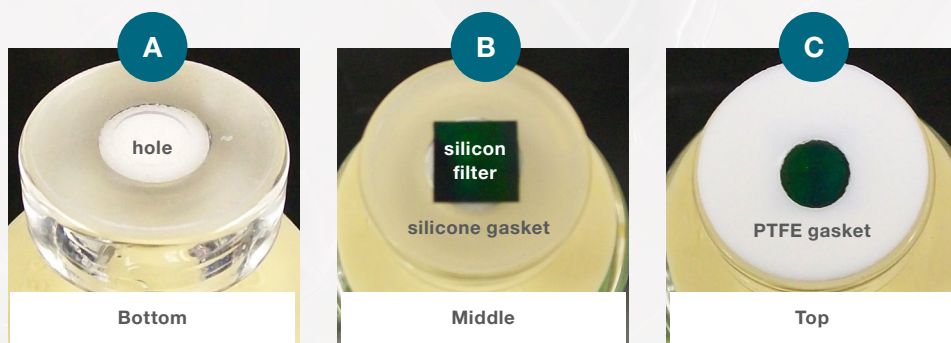
Figure 2: Setup of the gasket-filter-gasket system.
