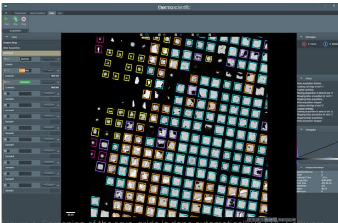
Figure 4. Screening of the cryo- grids is done automatically in EPU Software. Ice quality on the grids is grouped and color coded for easy assessment.
