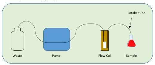
**NOTICE** Flow cells are connected so that the sample enters at the bottom of the chamber and leaves from the top. This arrangement is necessary to allow air to exit the chamber. If the cell were to be connected in the opposite direction an air pocket would be trapped in the top of the cell. Air bubbles or air pockets in the chamber cause incorrect and inconsistent absorbance readings to be recorded.
