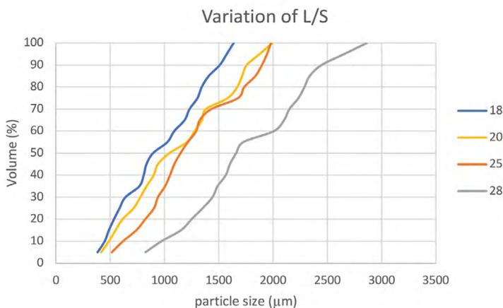
Understanding the influence of the liquid-to-solid ratio has on granule size.
