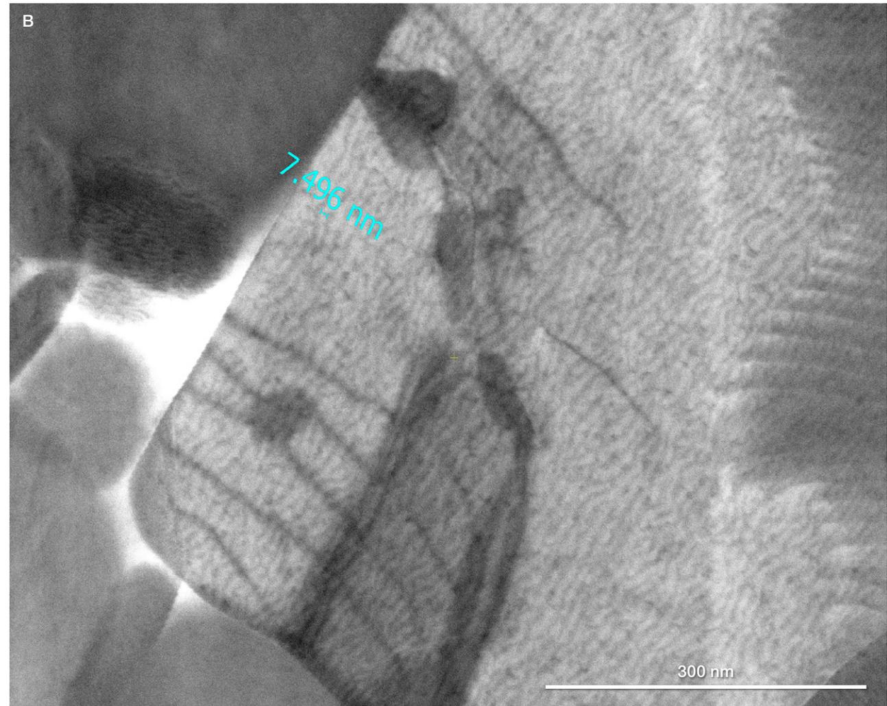
Figure 10. A) Transmission Kikuchi diffraction map shows the grain orientation of each individual sub-micron grain in an NMC cathode. B) High-resolution STEM imaging of a TEM lamella prepared from an NMC cathode.
