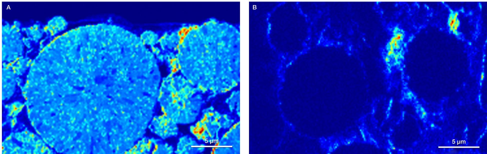
Figure 18. FIB-based ToF-SIMS maps of an NMC cathode cross-section. A)  $7\text{Li}^+$  map showing lithium distribution. B)  $19\text{F}^-$  map showing fluorine distribution in the binder.
