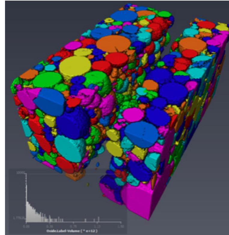
Figure 6. Illustration of the 3D analysis workflow using DualBeam Technology. Auto Slice & View Software was used for raw data collection followed by 3D reconstruction with Avizo Software.
