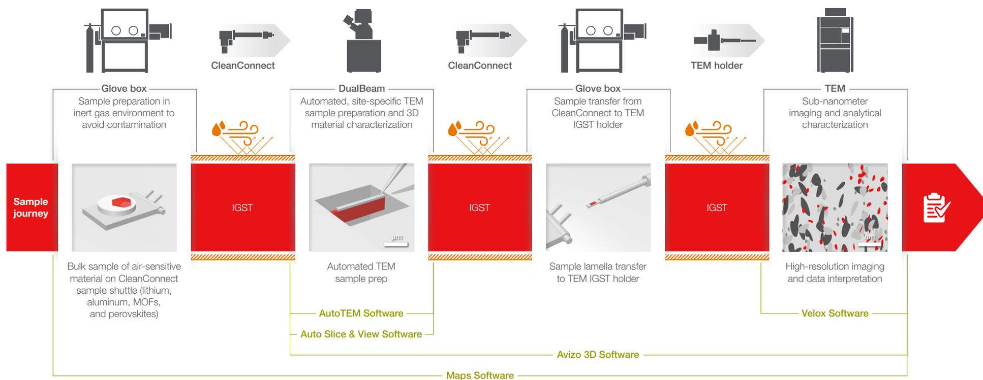
Figure 13. Inert gas workflow for nanoscale analysis, containing Thermo Scientific DualBeam and TEM systems.
