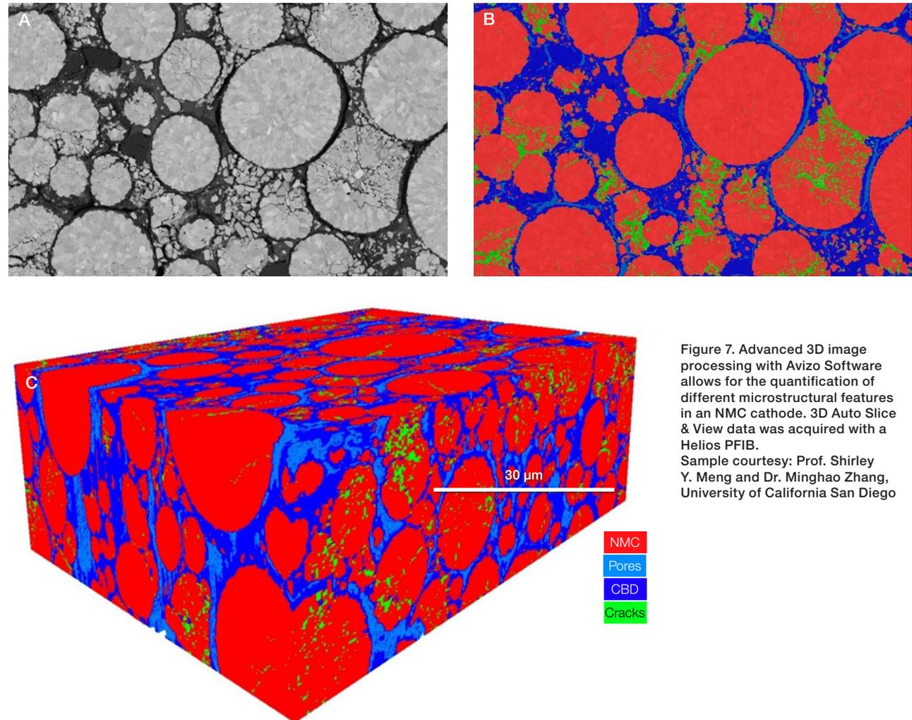
Figure 7. Advanced 3D image processing with Avizo Software allows for the quantification of different microstructural features in an NMC cathode. 3D Auto Slice & View data was acquired with a Helios PFIB. Sample courtesy: Prof. Shirley Y. Meng and Dr. Minghao Zhang, University of California San Diego
