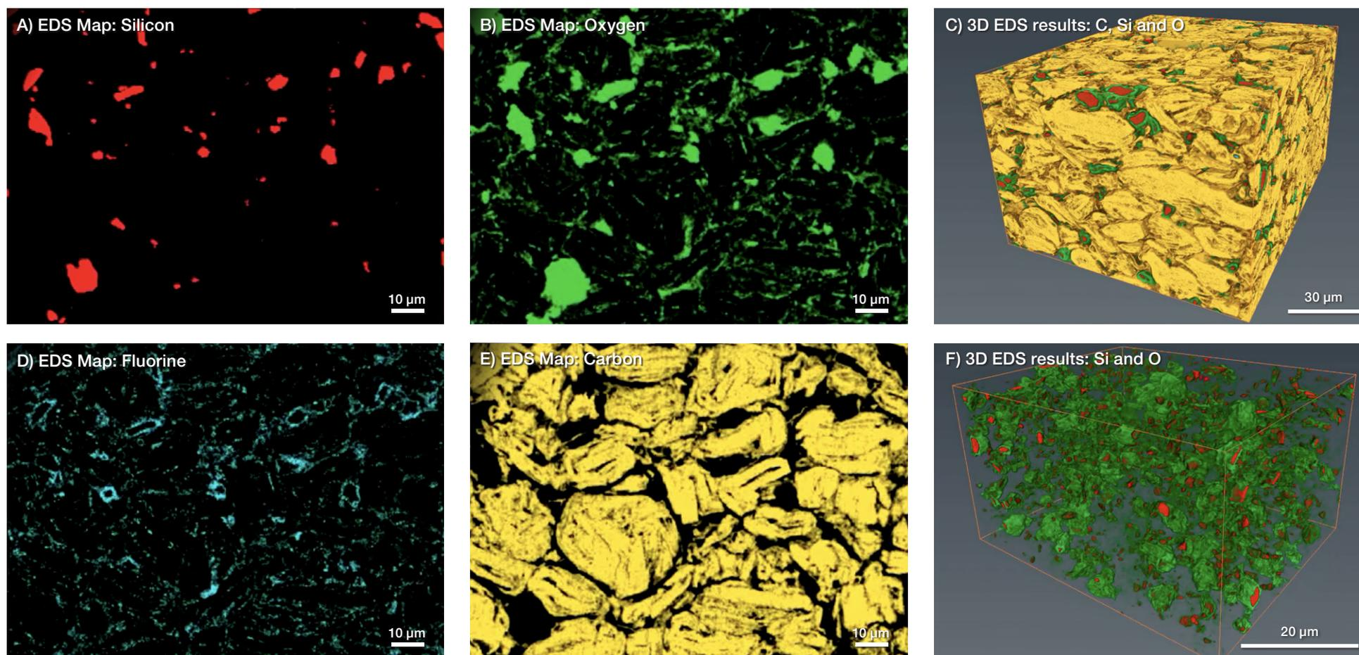
Figure 8. 3D EDS results showing the spatial distribution of CMC, PVDF additives and SiO particles in a graphite anode.
