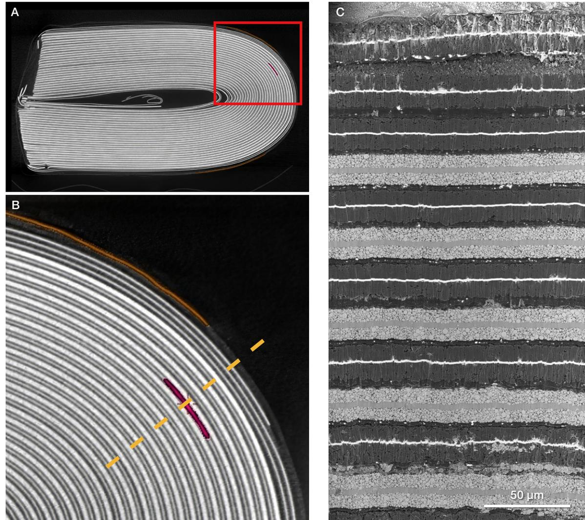
Figure 19. A) Overview image of the CT scan showing the location of the defect in the jelly roll battery. B) Defect (highlighted in red) identified with  $\mu$ CT, superimposed with a projected laser-cross-section plane (yellow dotted line). C) Laser-milled cross-section along the projected plane.
