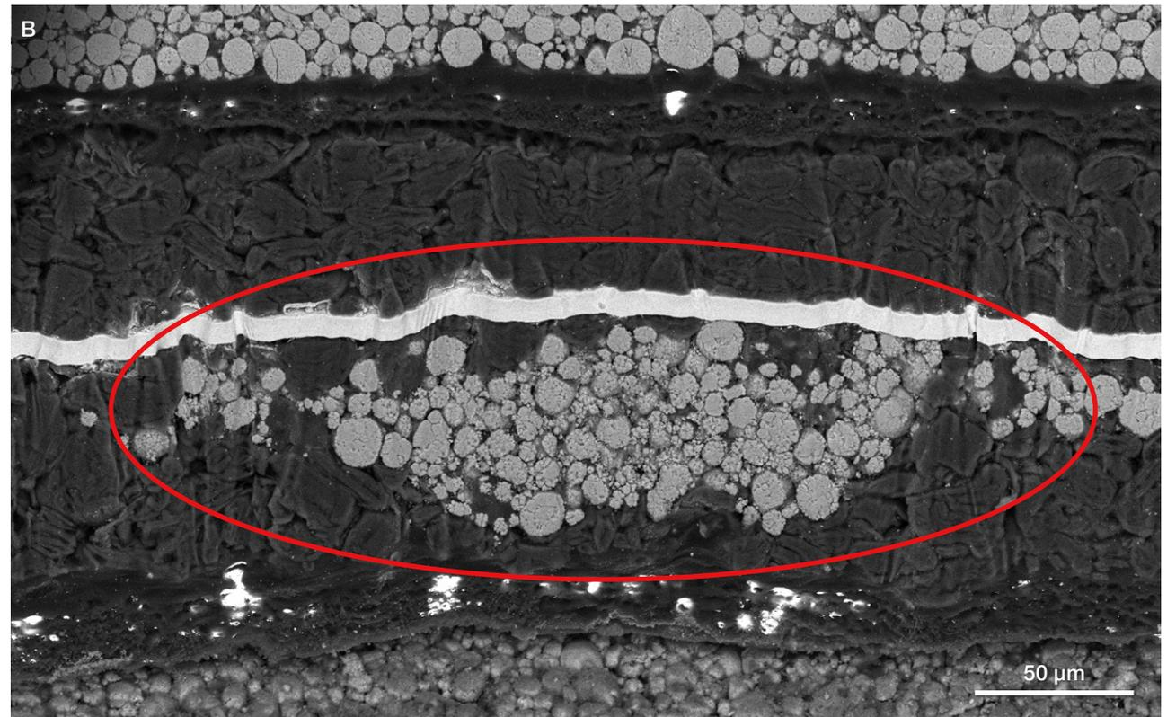
Figure 20. A) Overview of a large laser-milled cross-section showing a defect at the 11th layer of the battery cell. B) Close-up SEM image showing the morphology of the defect.
