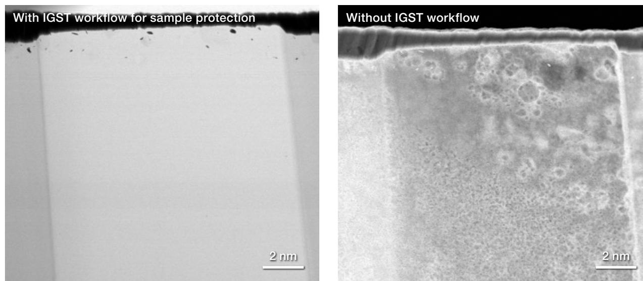
Figure 15. Li-metal lamella before and after 15 seconds of exposure in air.
