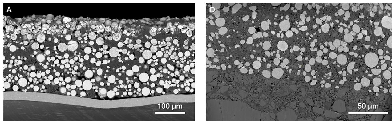
Figure 3. Various types of battery cathode cross-sections created and polished with DualBeam Technology. A) Li(Ni<sub>0.8</sub>Mn<sub>0.1</sub>Co<sub>0.1</sub>)O<sub>2</sub>. B) LiFePO<sub>4</sub>. C) A sodium battery cathode. D) A solid-state cathode with a sulfited solid electrolyte.
