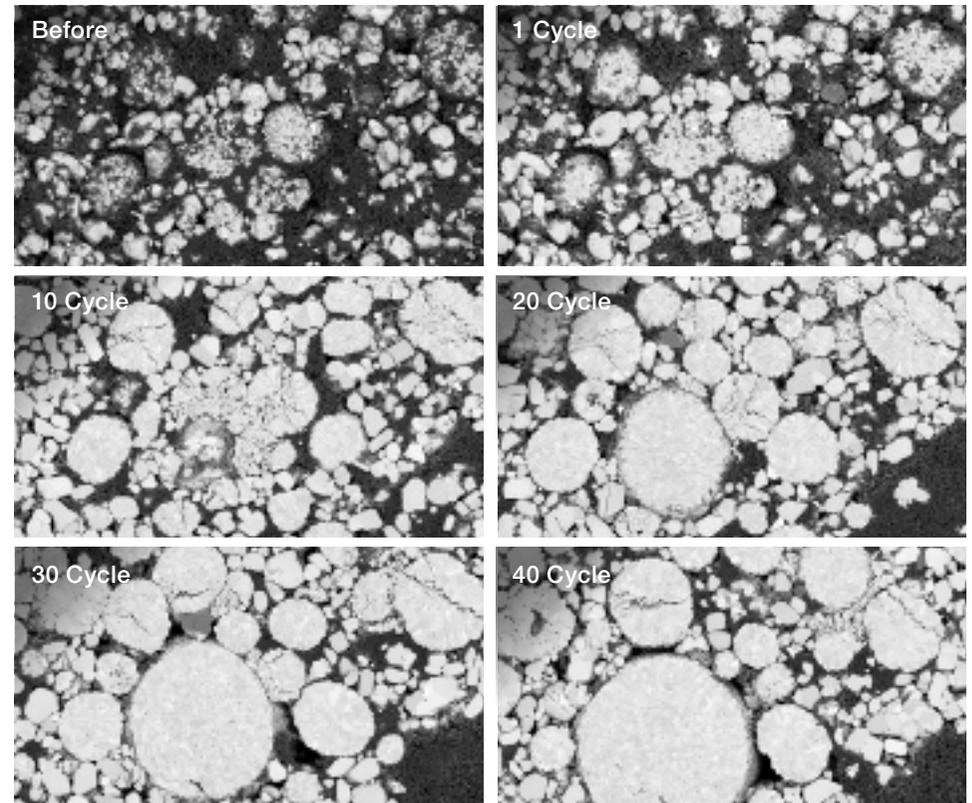
Figure 12. Spin milling analysis of a graphite anode and NMC cathode at various depths. Numbers indicate how many stage spins have been used to polish the sample.
