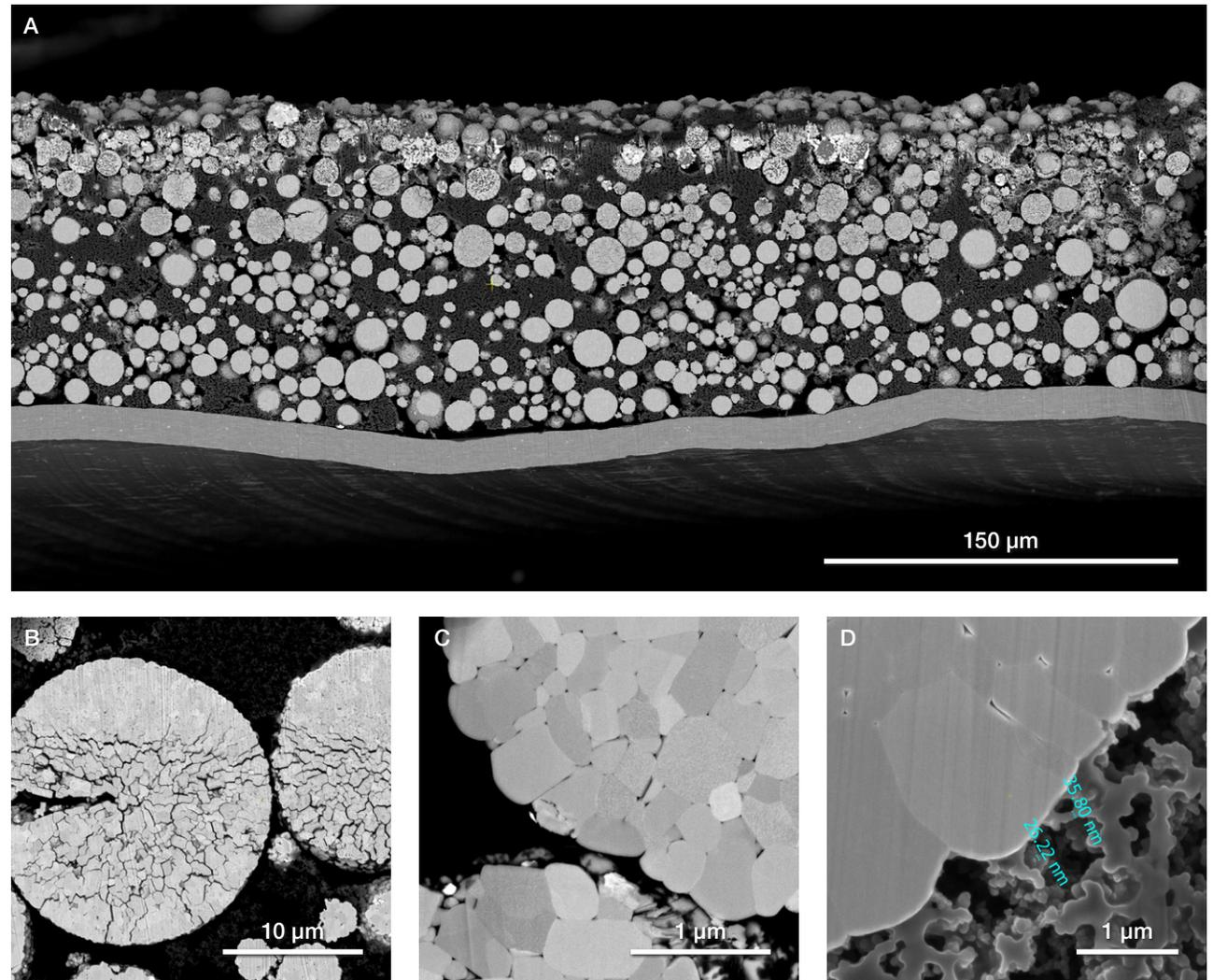
Figure 4. Multi-scale SEM images taken from a 600- $\mu\text{m}$  wide cross-section milled with a Helios PFIB, clearly resolving features from millimeter to nanometer scale.
