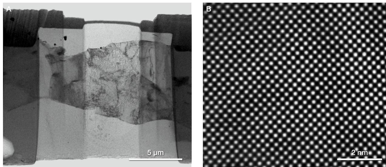
Figure 14. A) Li metal lamella with IGST workflow and B) Atomic-resolution TEM imaging of Li-metal atom columns. The IGST Workflow allowed the lithium metal lamella to stay crystalline with minimal signs of surface oxidation.
