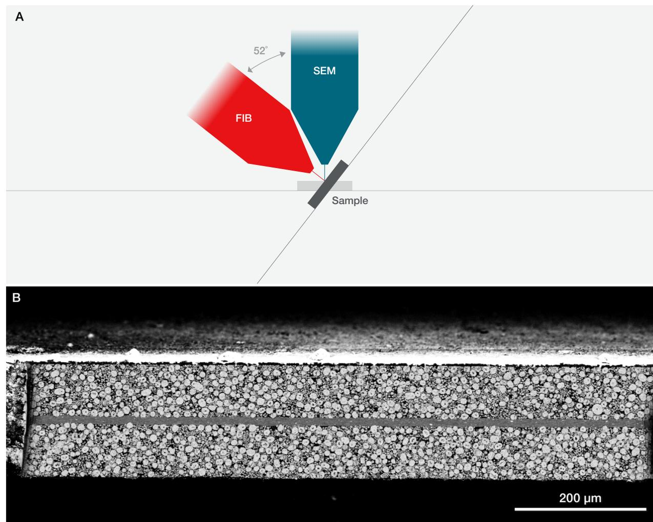
Figure 1. A) Graphical illustration of the DualBeam concept. B) 1,000- $\mu\text{m}$  wide cross-section of an NMC cathode.
