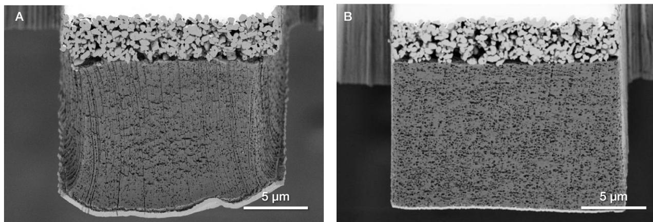
Figure 17. FIB cross-section of a cathode/separator film at (A) room temperature and (B)  $-80^{\circ}\text{C}$ .
