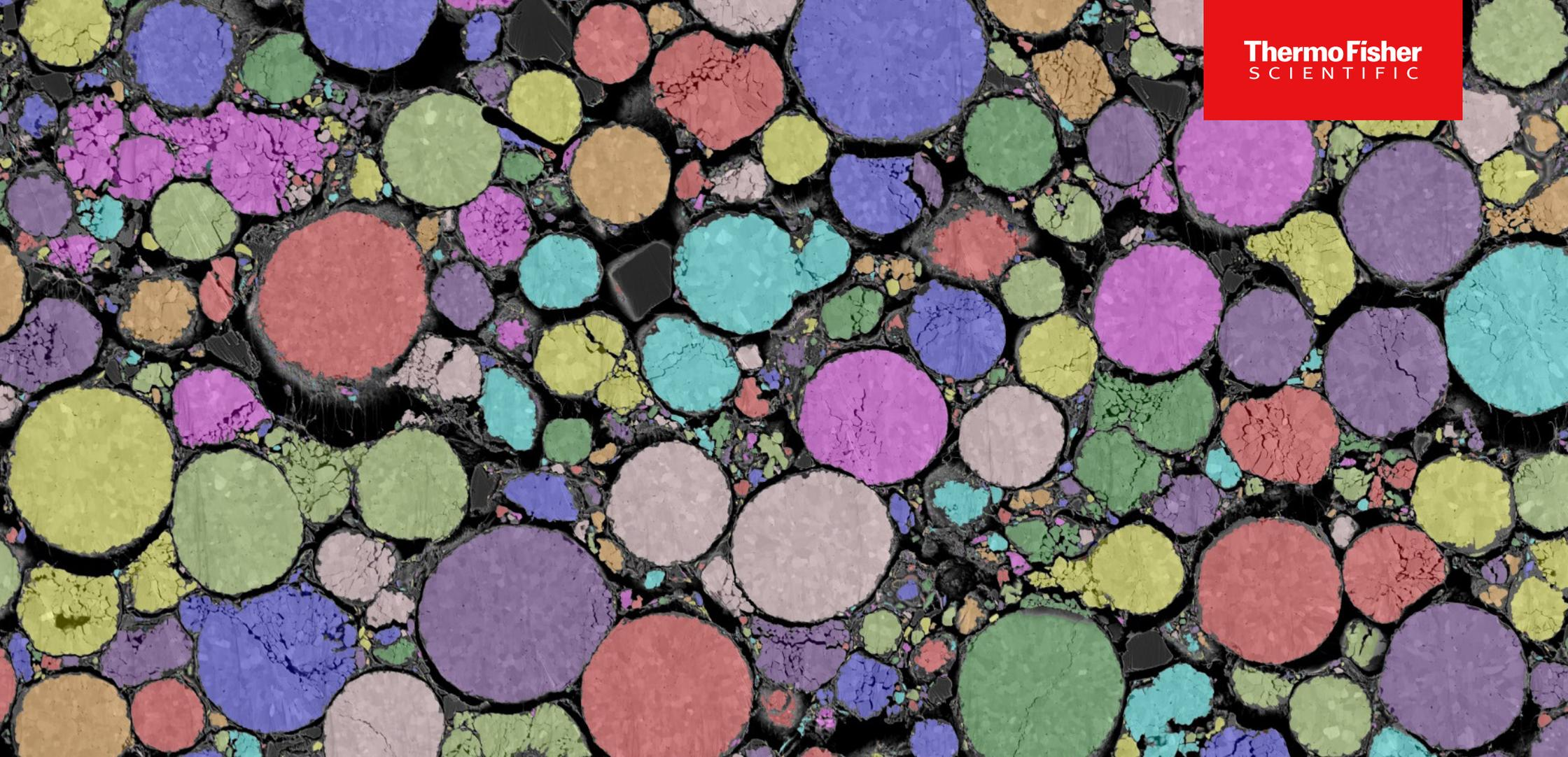
After cross-sectioning, multiple analytical techniques can be applied to a sample, including quantitative image analysis with Avizo 2D Image Processing Software, based on image contrast.
