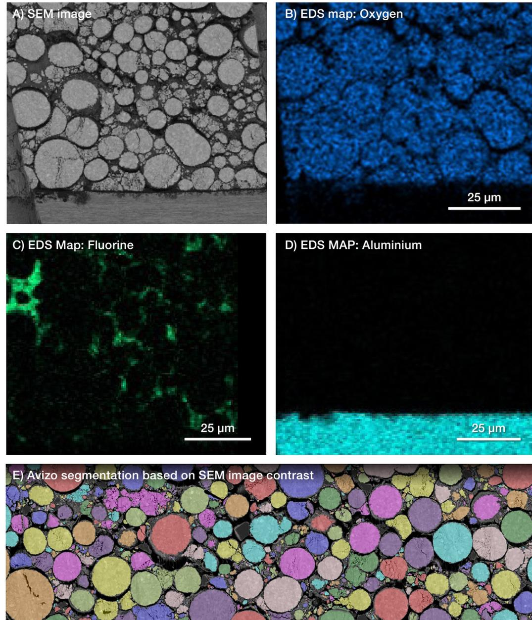
Figure 5. After *in situ* cross-sectioning (A), multiple analytical techniques can be applied to the sample, including elemental analysis with EDS mapping (B-D) or quantitative image analysis with Avizo 2D Image Processing Software, based on image contrast (E).
