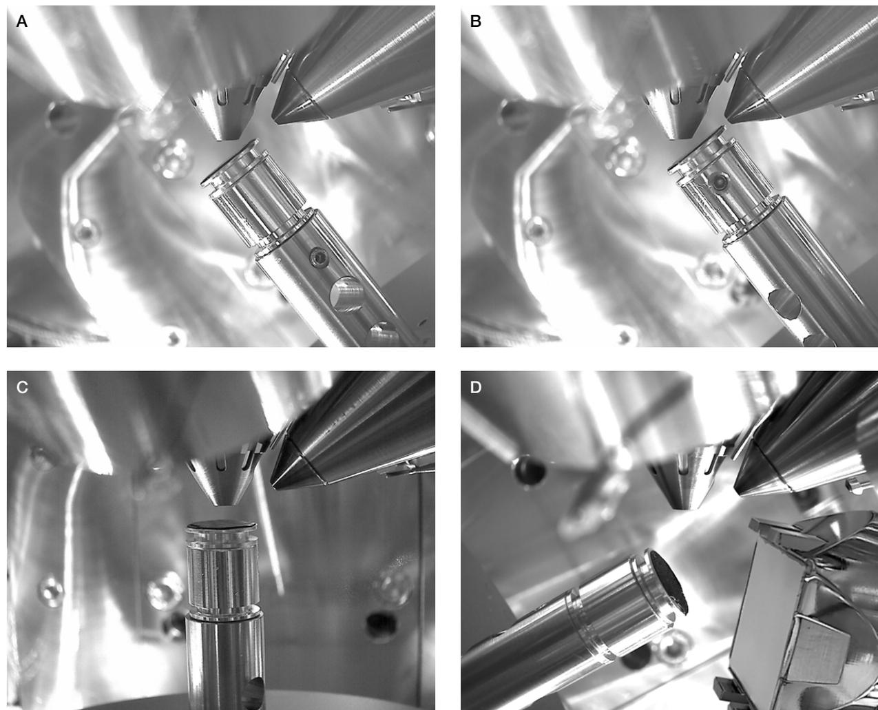
Figure 11. PFIB spin milling set-up for large-area sample preparation. Stage A) on-axis and B) off-axis compucentric rotation. C) SEM/EDS and D) EBSD data collection geometries.
