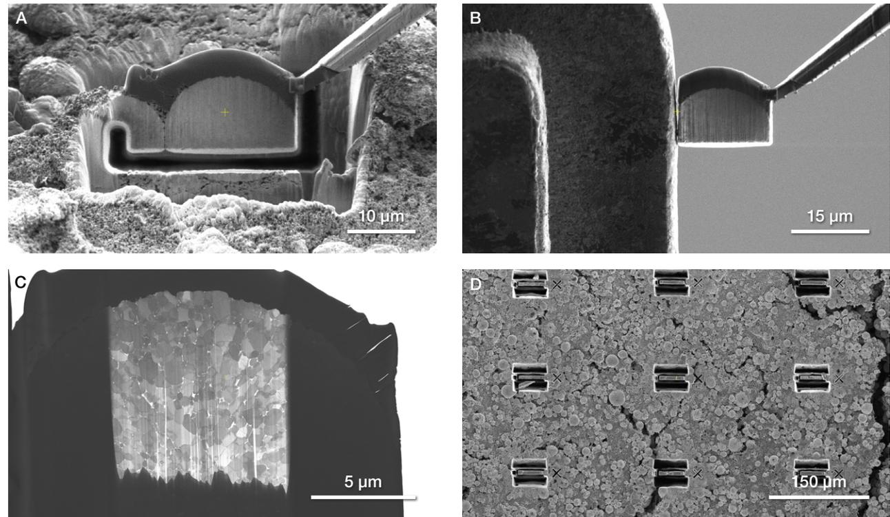
Figure 9. Automated TEM sample preparation from an NMC cathode with AutoTEM 5 Software. A) The lamella is prepared and is ready for lift out with the EasyLift Nanomanipulator. B) Automatic transfer to a TEM grid. C) Finally, the lamella is automatically thinned to electron transparency. D) Multiple lamella can be created from the bulk during the same workflow.
