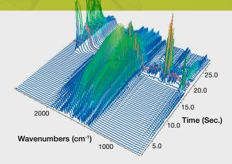
OMNIC Series software, unique Mercury TGA analysis package, and 3D displays allow you to quickly and efficiently extract useful information from TGA-IR (thermogravimetric infrared) and other time-based experiments
