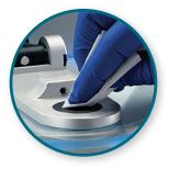
When the measurement is complete, the surfaces are simply wiped with a lint-free lab wipe before going on to the next sample.
