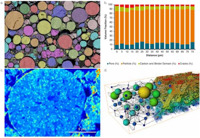
(a) and (b) NMC cathode cross-section prepared via Thermo Scientific Helios <sup>™</sup> 5 PFIB DualBeam and phase fraction analysis performed via Avizo2D Software; (c) TOF-SIMS analysis of the lithium distribution in NMC cathode; (d) 3D characterization of Li-ion battery graphite anode, data collected via Auto Slice & View 4 Software in Helios 5 Laser PFIB; structural quantification performed via Avizo Software.
