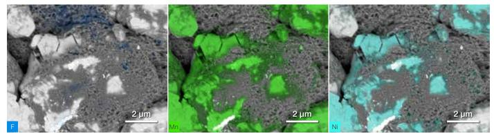
Apreo SEM and ChemiSEM Technology analysis of a Li-ion battery cathode surface using real-time EDS.
