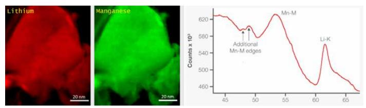
EELS spectrum images of Li battery materials. The Mn-M edge fine structure and Li-K edge in the Li battery are distinguished with an energy resolution of <0.28 eV. Results were collected on a Thermo Scientific Talos<sup>™</sup> F200 (S)TEM with X-CFEG, Panther STEM, and Gatan Continuum 1066 at 200 kV. Sample courtesy Dr. Chongmin Wang, PNNL.
