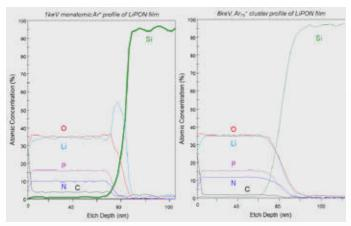
Depth profiling analysis of the LiPON solid electrolyte to understand the stoichiometry of the film as a function of depth. The 1 keV monatomic profile induces Li "pile-up" at the interface as defects while cluster profile induces Li "pile-up" at interface.
