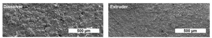
Left: Cathode slurry mixed using a dissolver. Right: Cathode slurry mixed using a twin-screw extruder.
