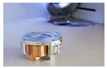
Vacuum transfer module for sample protection.
