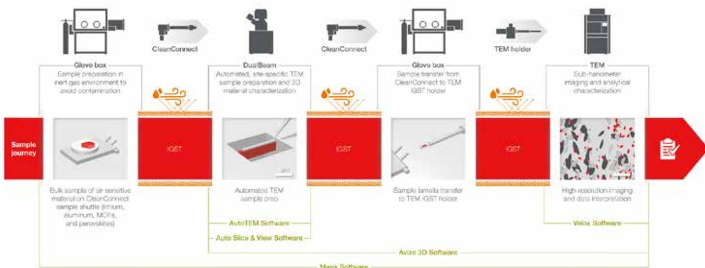
IGST Workflow using Thermo Scientific scanning electron microscopes.
