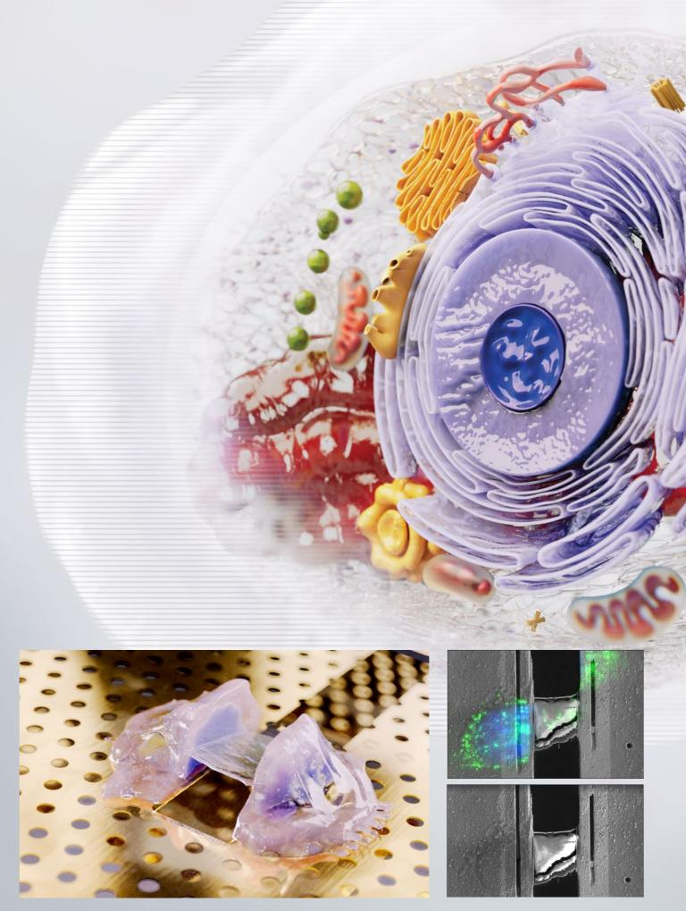
Fluorescence imaging for targeting, intermediate verification, and final target confirmation can easily be done before, in-between, and after ion milling without moving the stage.
