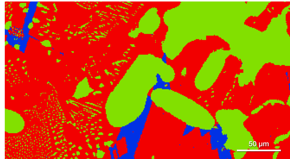
Characterization of a zirconia mullite sample with ChemiPhase. Phase analysis shows the presence of an unexpected contaminant phase rich in silicon and sodium. Thanks to ChemiPhase, the composition and quantification of each of the phases has been obtained with a click. Acc voltage 15 keV, beam current 0.48 nA.
