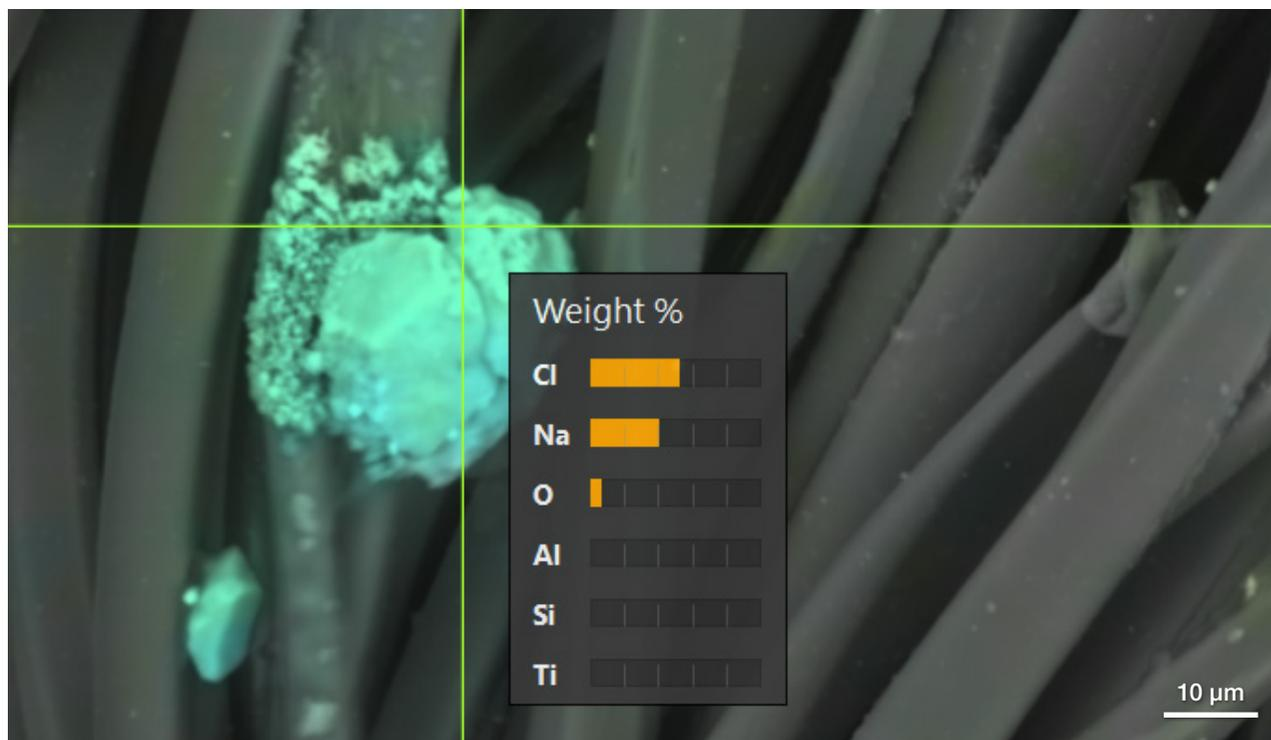
Figure 3. Live view of the SEM user interface showing a ChemiSEM image of unknown materials on a used face mask. The tooltip shows the composition of one of the regions, making it easily identifiable as sodium chloride, hence not a harmful contaminant.
