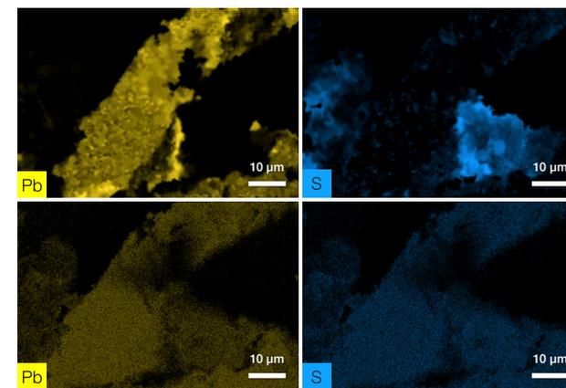
Figure 12. ChemiSEM Quantitative Maps (top) and conventional gross counts maps (bottom). Both conventional gross count maps are based on a signal coming from one peak and are therefore the same.
