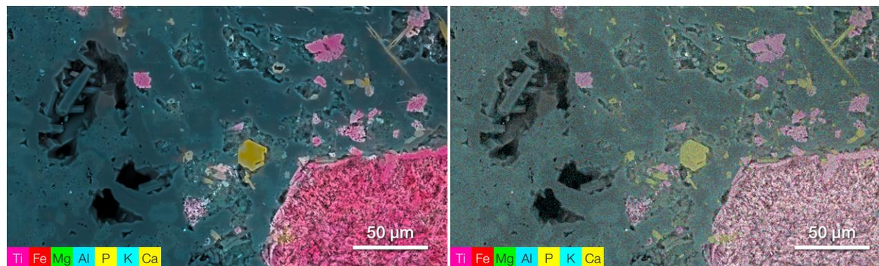
Figure 2. ChemiSEM image (left) and gross counts mapping (right) of contaminants on a battery anode.
