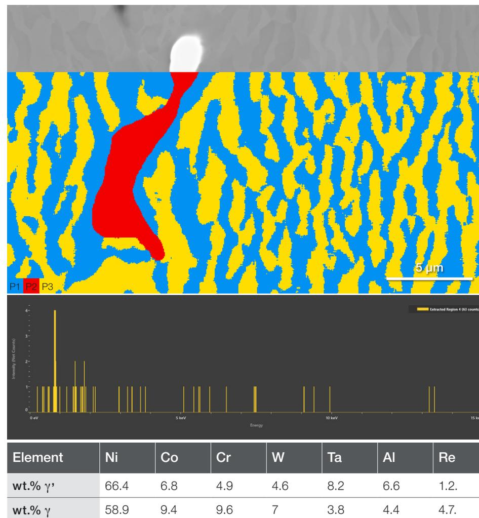
Figure 13. ChemiSEM phase identification in a Rene N5 Ni-based superalloy. The image shows a tantalum carbide in the base alloy, which is made of two phases: gamma (blue) and gamma prime (yellow). ChemiSEM quantification of each of the phases was calculated from only 30 average counts per pixel, as shown in the extracted point spectrum from the gamma phase.
