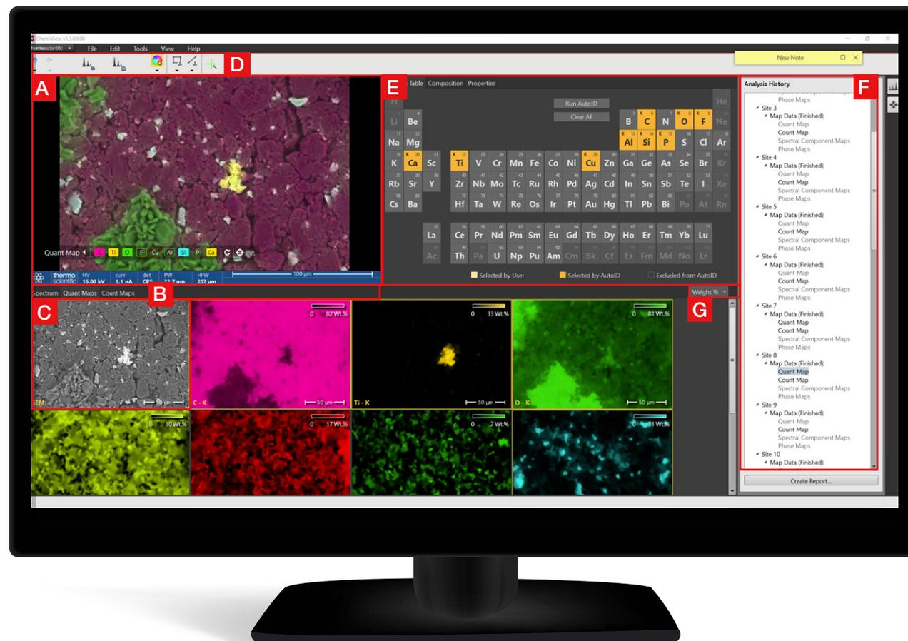
Figure 1. ChemiSEM user interface showing combined SEM-EDS operation in a single display.
