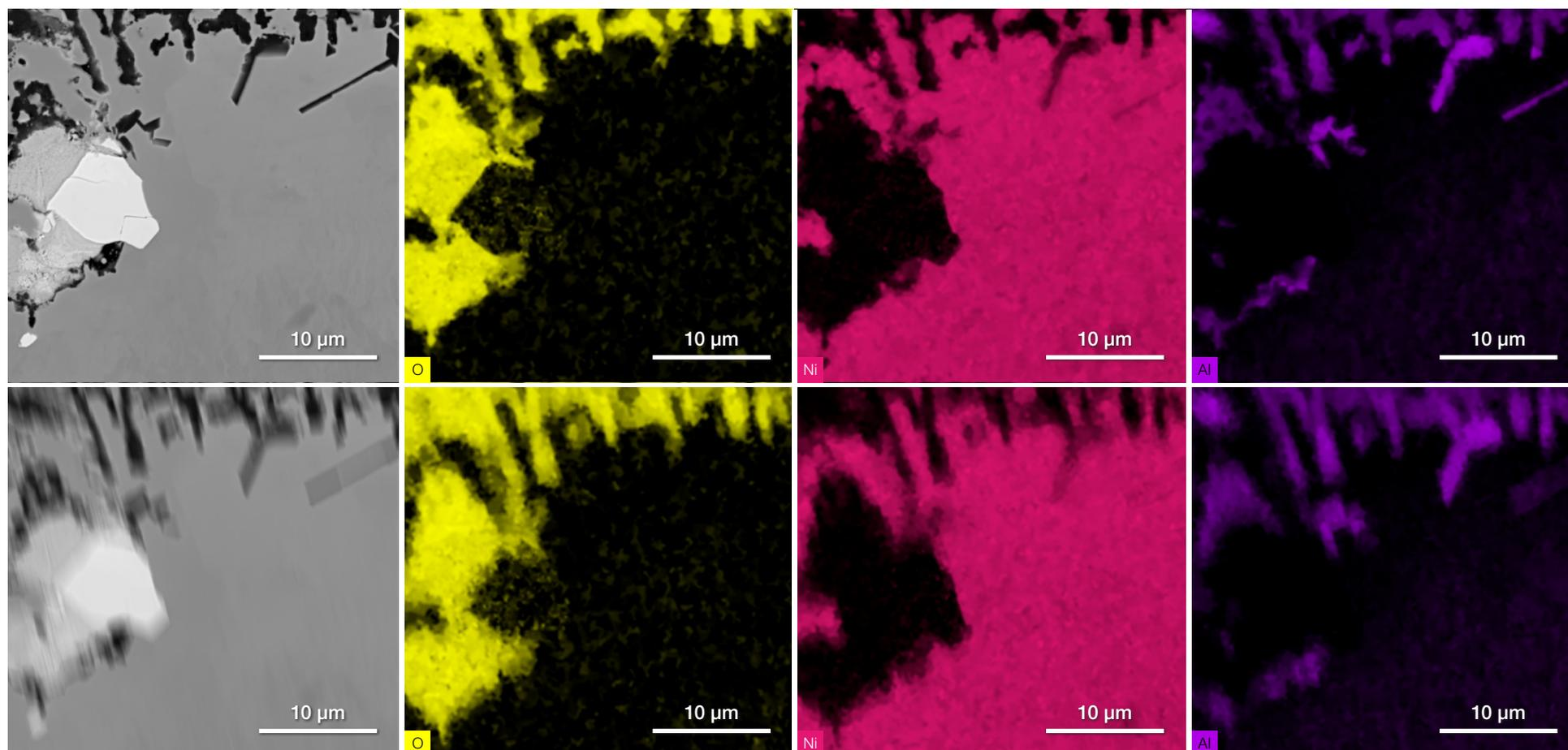
Figure 14. Rene N5 superalloy cross section showing surface damage and oxidation from thermal cycling. Top: drift corrected. Bottom: no drift correction.
