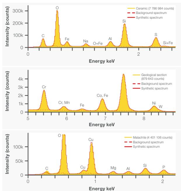
Figure 6. Examples of spectra acquired from a ceramic (top), a geological section (middle), and a polished section of malachite (bottom) under different acquisition conditions. In all cases, both background (dotted line) and synthetic spectrum (red line) can be seen. The ways in which simulated spectra fit with experimental data are clearly visible regardless of the acquisition condition and material, confirming the high quality of the processing.
