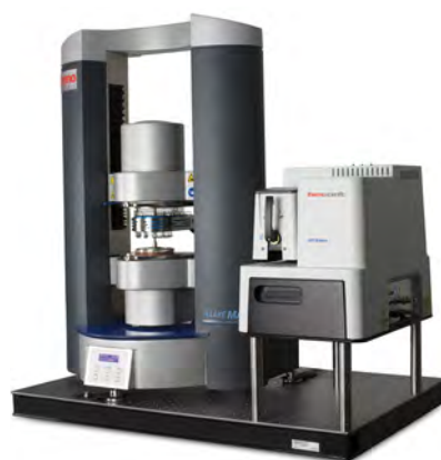
Figure 1: The Thermo Scientific HAAKE MARSxR RheoRaman system.
