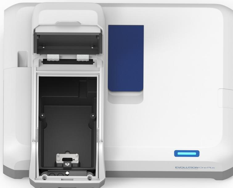
**Note** Ensure the tubing does not obstruct the light beam or prevent the sample compartment door from closing. If necessary, secure the tubing using the supplied clips.
