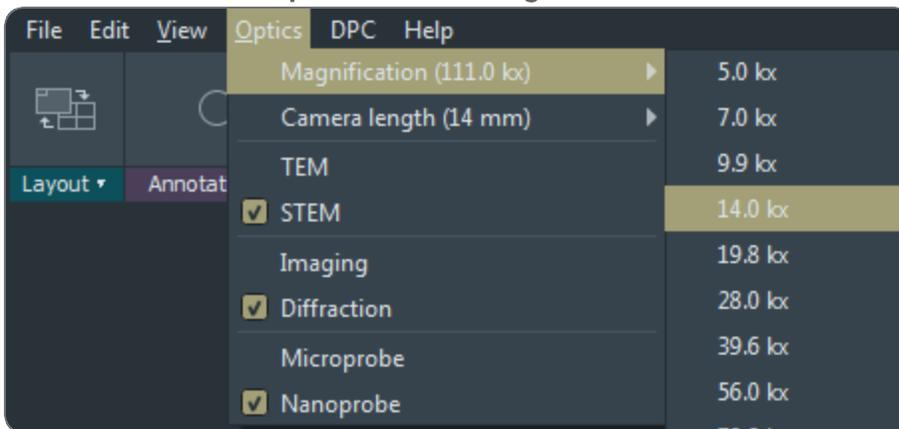
In STEM Imaging mode, the Optics menu does not offer the *Field of View* parameter. Instead it offers a set of *Magnification* values, where  $\text{Magnification} = 0.1 / \text{Field of view}$  with the assumption that the width of the field of view is 10 cm.
