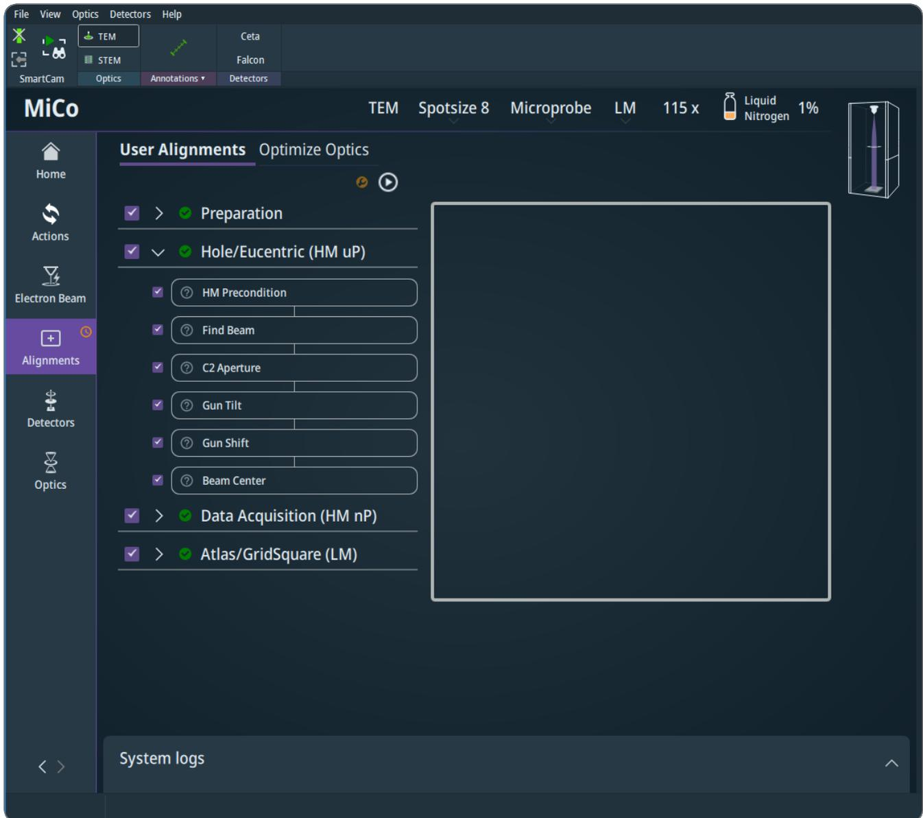
It should be noted that the microscope state is automatically saved upon successful completion of each complete alignment sequence. In case of a failure for one or more modules, it is possible to manually perform these alignments using TEM User Interface. In such case, it is recommended to save the state (wrench icon) of the microscope manually after finishing.
