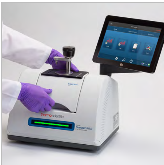
Figure 2-3: Lowering an accessory into place on a Nicolet Summit PRO.
