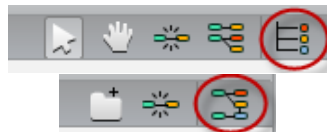
Figure 18.58: 1: Switch to the Project Tree View - 2: Go back to the Project Graph View
