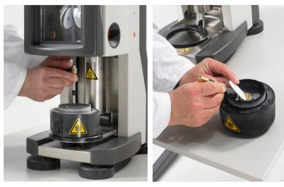
It is recommended to remove the access of liquid ethane – that may be capillary present in the groove of the tweezers that hold the grid – with some filter paper. The anti-contamination ring, which floats on the liquid nitrogen, creates a cold gaseous atmosphere which facilitates the transfer and minimizes possible ice contamination on the grid. The outer ring contains a circular storage grid box for four grids underneath a layer of liquid coolant gas.
