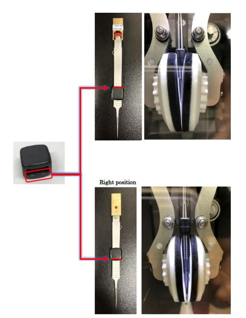
Mount the tweezer onto the connection grove in the central axis. To do this, first select the 'Place New Grid' button in the Vitrobot User Interface to put the central axis in the right position for mounting the tweezer to it.
