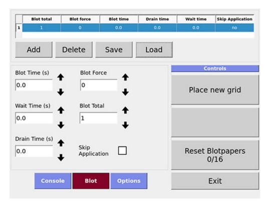
In the **Blot** screen, additional vitrification parameters can be set. For example the relaxation time before the blotting (Wait Time) and the intermediate time between blotting and plunge freezing (Drain Time).
