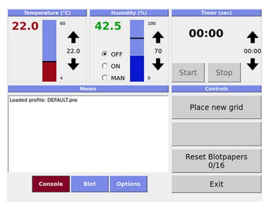
In the **Console** screen the temperature can be set towards any value between 4 °C and 60 °C with the + and – buttons or drag the black marker up or down. The actual temperature read-out is displayed in red.
