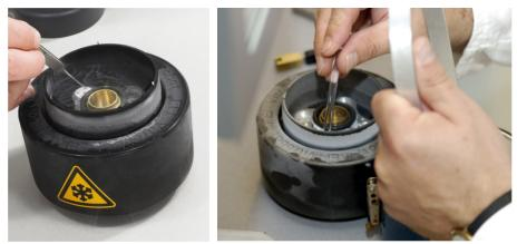
After the grids have been transferred into the grid box, they are sealed with a special screw and usually stored into a somewhat larger dewar for liquid nitrogen prior to the transfer into a cryo holder and subsequently a TEM or SEM.
