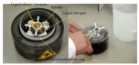
When the ethane/propane container is ready for vitrification the holder can be placed on the platformring under the Vitrobot.
