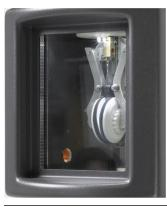
**Note** After a maximum of 16 blottings, the filter papers must be replaced. The UI displays the message: 'Replace Blotpapers'.
