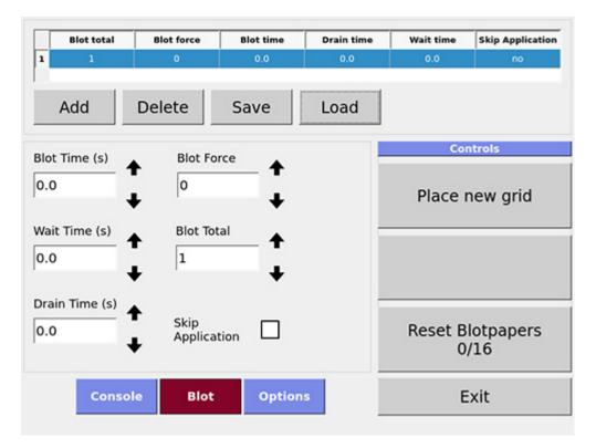
For manual application of the sample onto a grid, select with the foot pedal switch or the stylus 'Continue' to proceed. The tweezers is slightly lowered as to allow the application of suspension through the side-entry port using a pipette. As a consequence of this method only one side of the grid is inoculated with suspension. The advantage of this method is that only small volumes of the sample (typically 3  $\mu$ I) are used.
