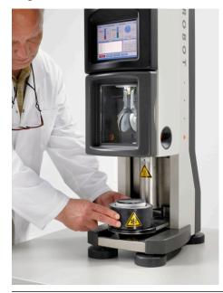
**Note** Make sure that liquid nitrogen remains present in the peripheral ring throughout the entire vitrification procedure.
