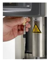
The tweezers with grid are subsequently lifted into the climate chamber by selecting the 'Start Process' button in the User Interface, or alternatively, use the foot pedal switch. The environmental and process parameters (i.e. temperature, humidity, number of blots etc) can now be set as described in: Starting Up – Switching on the Vitrobot on page 14
