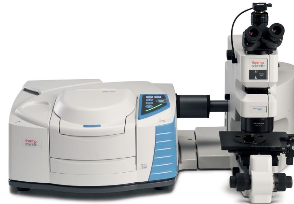
System configured with high sensitivity liquid nitrogen cooled MCT detector
