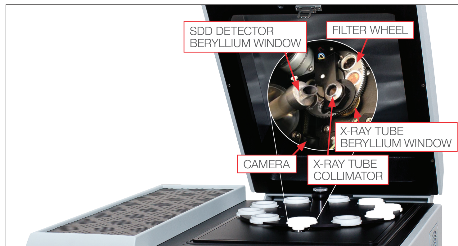
Different components of the EDXRF spectrometer
