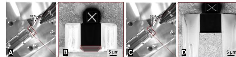
Orientation of the sample surface with respect to the PFIB/SEM columns. (A) Position of the stage and sample during the milling process. Cross-section is milled with the ion beam perpendicular to the sample surface. (B) Ion beam view with illustrated sequential milling of the selected prepared area (20 µm). (C) The stage at imaging position with the sample surface kept perpendicular to the ion beam. (D) Exposed cross-section area of the mouse brain tissue embedded in EPON resin.
