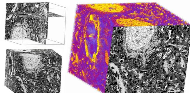
Sample volume of region of interest using cross-section technique. Oxygen (30 kV, 0.61 nA) was used to mill 10-nm-thick slices. Image taken with thought lens backscattered detector at 2 kV. Selected slices along the XY, ZX, ZY planes. 3D reconstructed volume, segmented to reveal structural details. Total volume = 23.4 µm x 18.2 µm x 20.0 µm. Mouse brain tissue embedded in LR White resin
